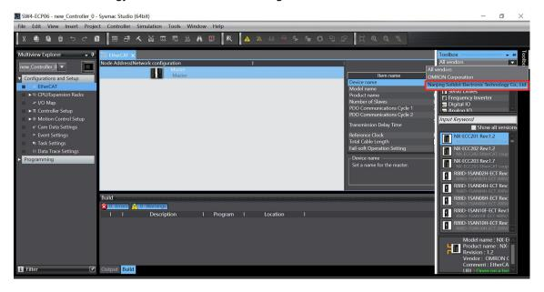
b. Click to select EtherCAT Infrastructure component, double-click the SW4-ECP06 module, and add a slave device, as shown in the following figure.
