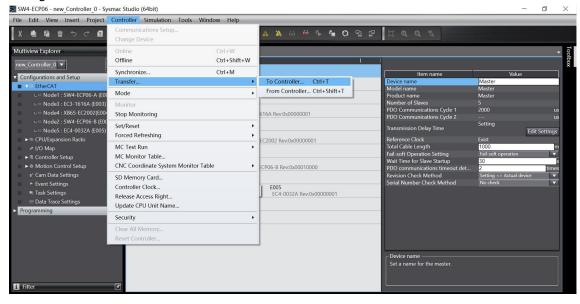
b. Download the configuration to the PLC, as shown in the figure below. After the download is complete, you need to power on again.
