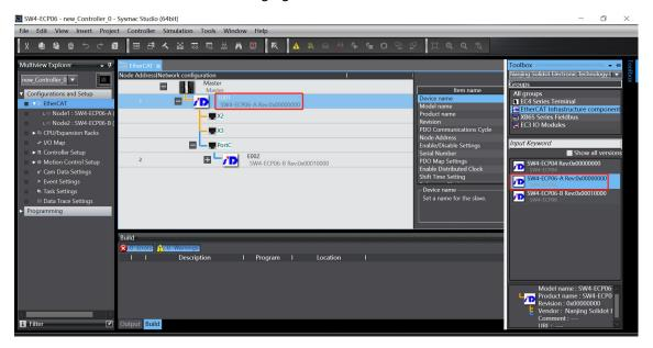
c. Add other modules according to the actual connection topology, as shown in the following figure.
