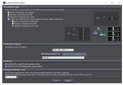
d. Click Ethernet Communication Test. The system displays that the test is successful.
