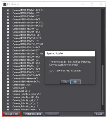
d. Click the "Install (File)" button again, select the XML file paths of other modules in the topology configuration and install them one by one. In this example, select the EC3 configuration file path and click the "Yes" button to complete the installation, as shown in the following figure.
