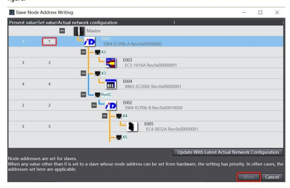
f. After writing, a power-on prompt pops up, as shown in the figure below. Click the "Write" button and restart the slave device power according to the prompt.
