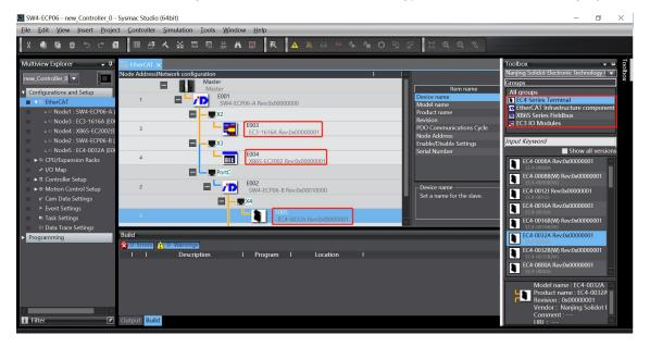
d. Click "Controller->Online" in the menu bar to switch the controller to online status. Right-click the master device and click "Write Slave Node Address", as shown in the figure below.
